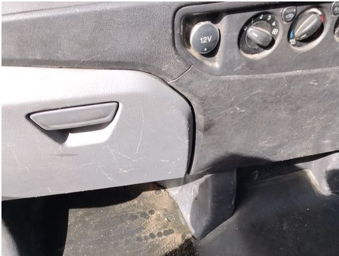
19: Centre Console Front Scuffed Over 25mm
