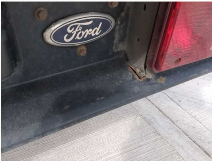
11: Bumper Rear Cracked Over 25mm
