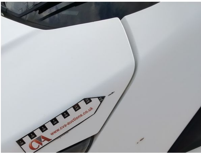
3: Bonnet Scratched Over 25mm Thru Paint
