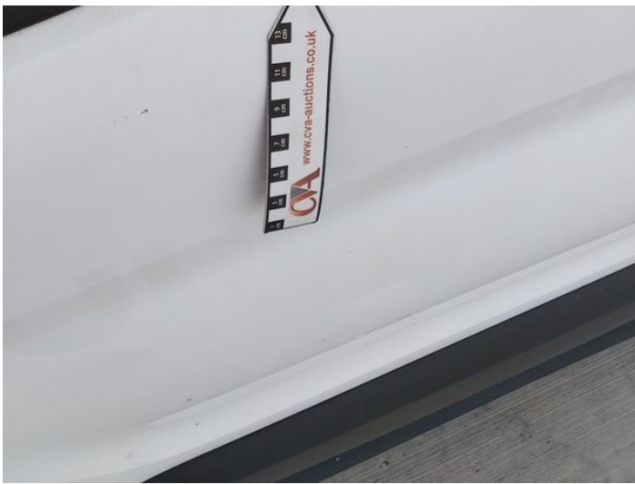
9: Door nsf Rusted UpTo 5mm
