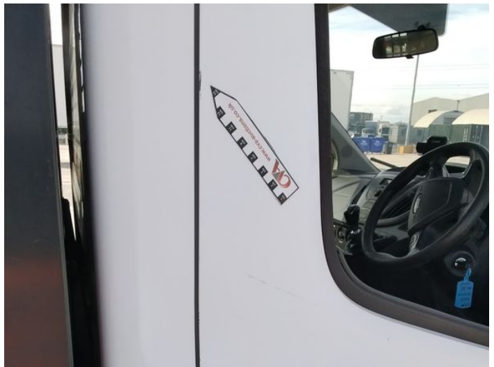
12: Door osf Chipped Multiple Chips
