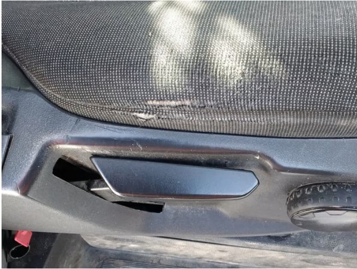
17: Seat Base Cover osf Torn Over 3mm
