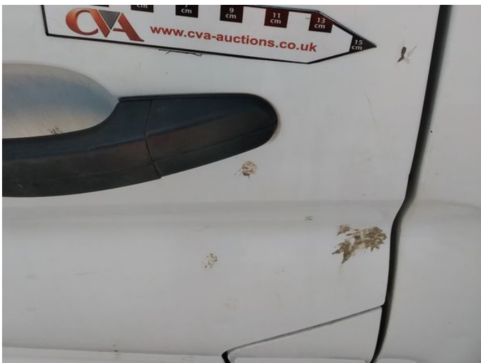
7: Door nsf Scratched Over 25mm Thru Paint
