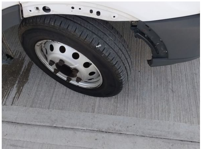
14: Wing Front Arch Extension os Missing Replace
