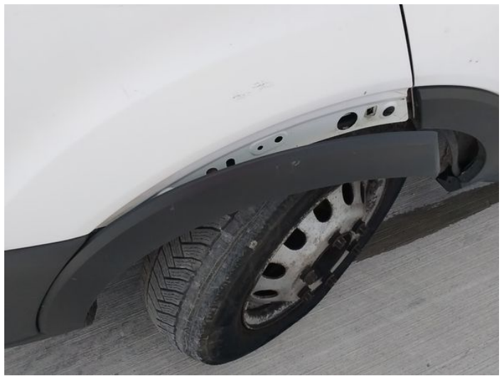
4: Wing Front Arch Extension ns Broken Replace
